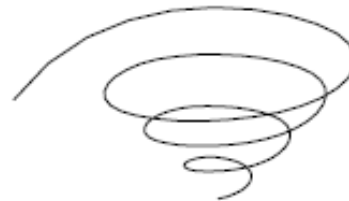
3D polyline after curve-fitting
