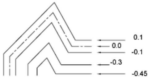
a four-element multiline, each element offset from 0.0
