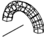
circle path curve divided into equally sized intervals
