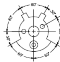
text aligned with and centered within the dimension line
