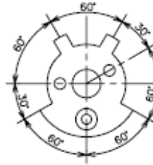
ISO standard text above the dimension line
